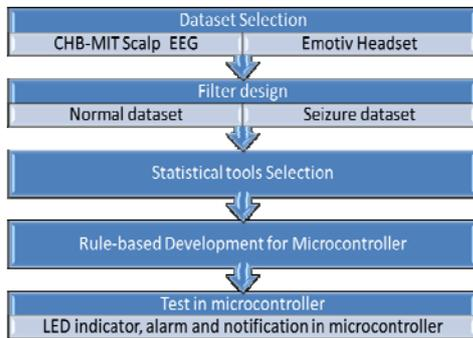
Figure 2. Flowchart of the Wearable Computing System for the Seizure Detection.
