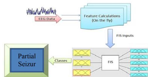
Figure 9. Block Diagram of the Fuzzy Engine System.
