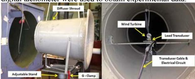
Figure 15. Laboratory Setup for Enhancement of Power Augmentation
