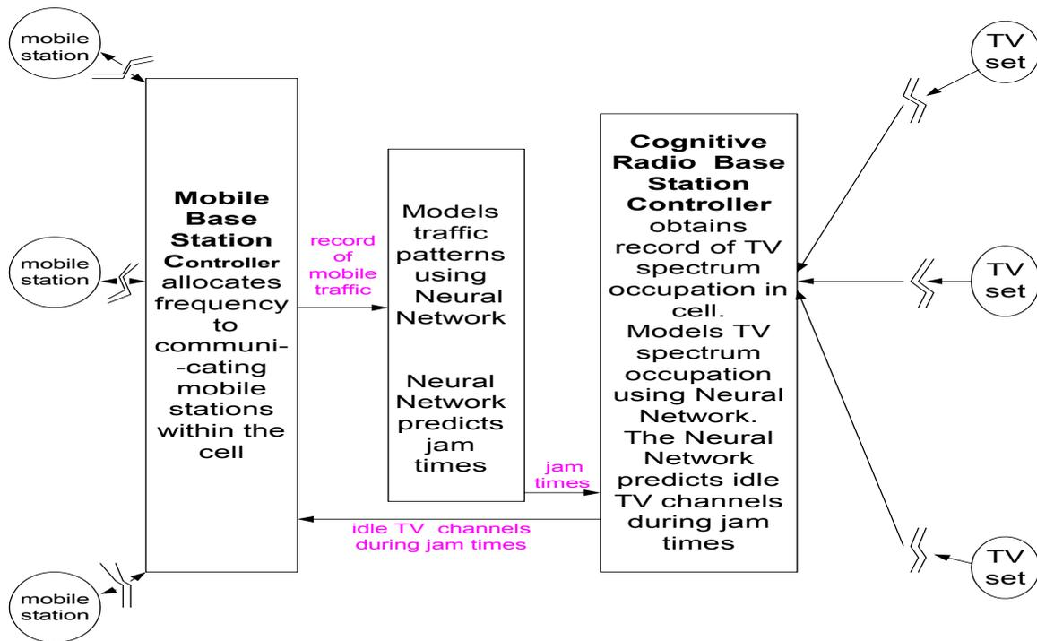
Fig. 1 - Model to Enable TV Receiver Spectrum Holes to be Used to Serve Over-burdened Cellular Networks
