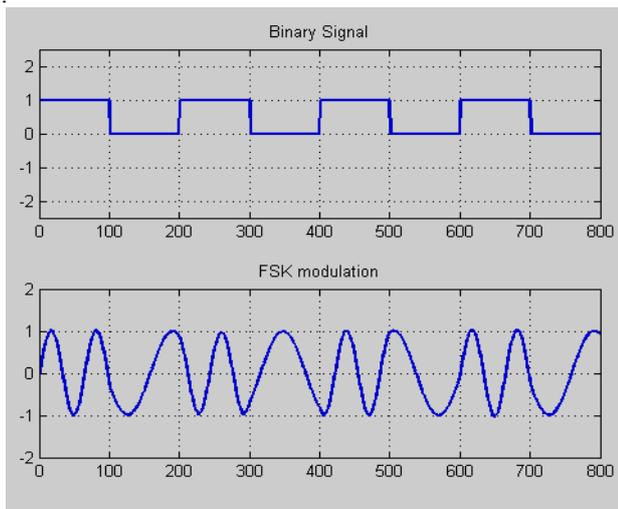
Fig.4 FSK application of proposed oscillator
