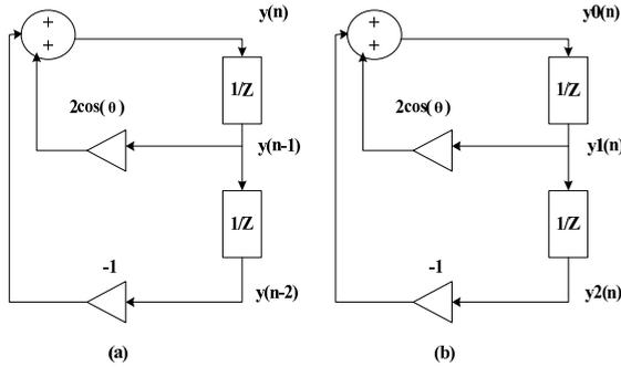
Fig. 1 (a) The Structure of sine oscillator, (b) The structure of cosine oscillator
