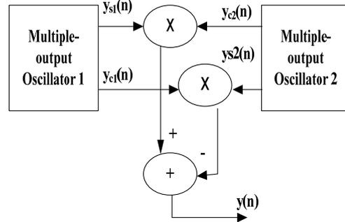
Fig.3 The complete oscillator structure
