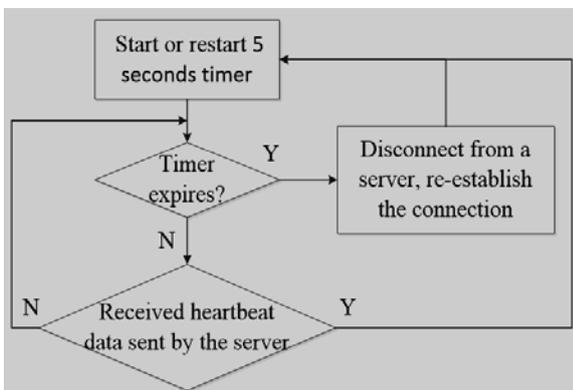
Fig. 3. Flowchart of Heartbeat Mechanism
