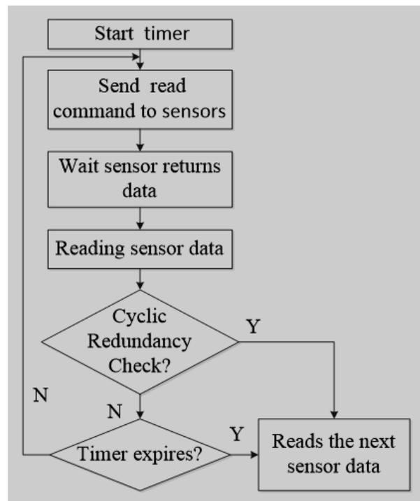
Fig. 4. Flowchart of Reading Sensor
