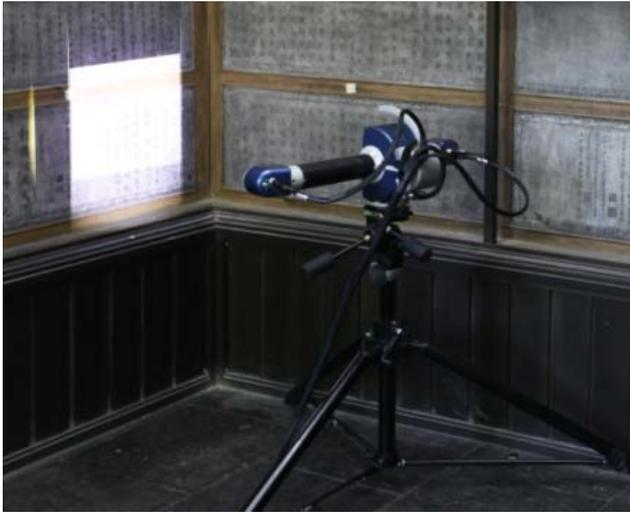
Figure 5. Structured-light scanner project a pattern of light on stone tablet, then calculate 3D data.
