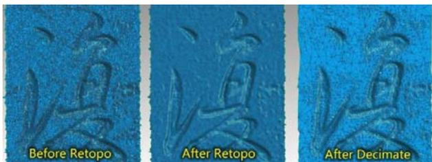
Figure 8. Retopo produces a uniform tessellation of mesh, and decimate will make data convenient to use.
