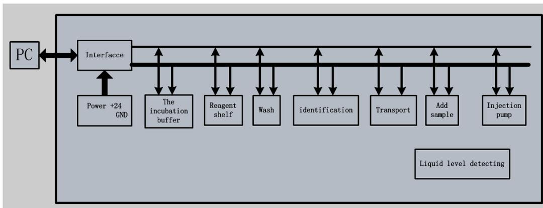
Fig.1 System function module chart
