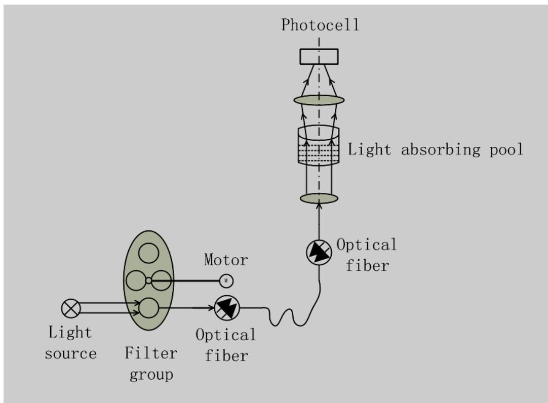
Fig.3 Optical system diagram
