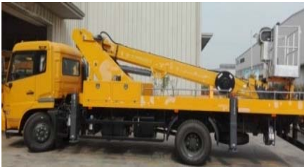
Figure 12. A typical aerial work platform
