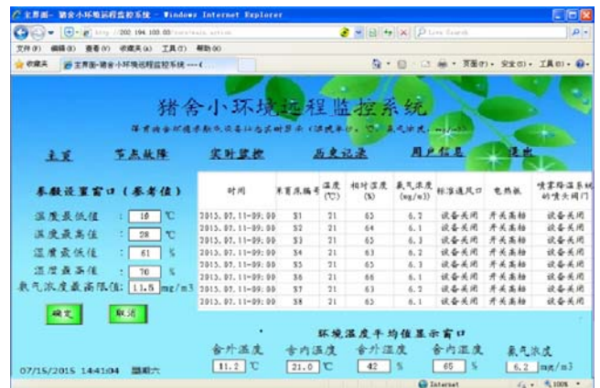
Fig.11 Browser-based User Interface of Environmental Monitoring and Control System
