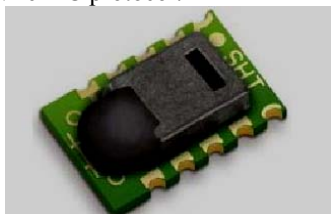
Fig.4 Temperature Humidity Sensors
