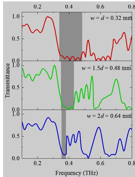
Figure. 7 Transmission spectra of PCMP with  $l = 0$  and different  $d$  ( $d = 0.64\text{ mm}$ ,  $d = 0.48\text{ mm}$ ,  $d = 0.32\text{ mm}$ ).
