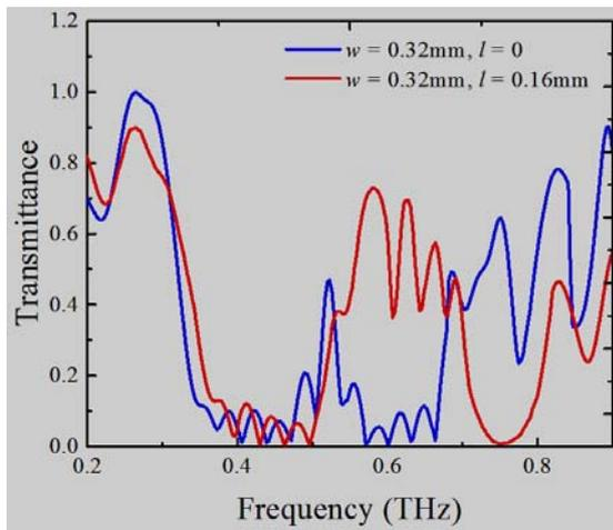
Figure. 8 Comparison of measured transmission spectra of PCMP with  $w = 0.32 \text{ mm}$ ,  $l = 0$  and  $w = 0.32 \text{ mm}$ ,  $l = d/2 = 0.16 \text{ mm}$
