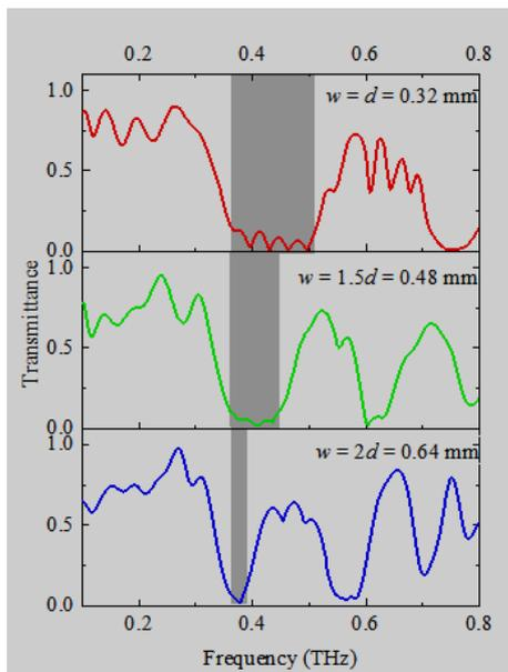
Figure. 9 Transmission spectrum of PCMP with  $l = d/2 = 0.16 \text{ mm}$  and different  $d$  ( $d = 0.64 \text{ mm}$ ,  $d = 0.48 \text{ mm}$ ,  $d = 0.32 \text{ mm}$ ).
