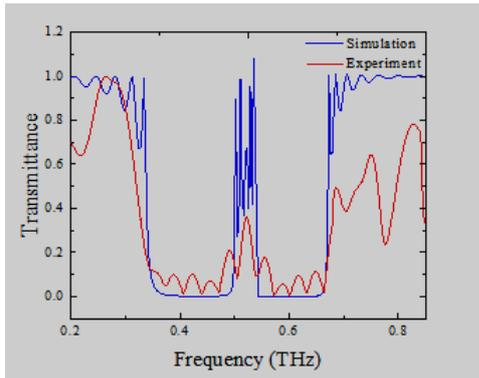
Figure. 6 Measured and simulated transmission spectra of PCMP with  $w = 0.32\text{ mm}$ ,  $l = 0$ .
