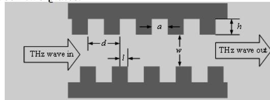
Figure. 1 Schematic structure of the PCMP and its corresponding geometry parameters.
