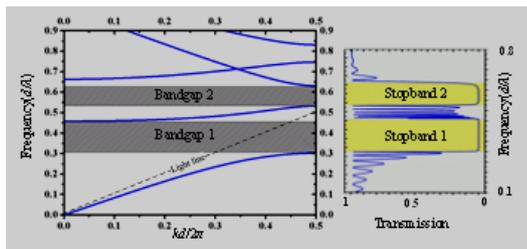
Figure. 2 Dispersion relations of PCMP ( $l = 0$  mm,  $w = 320$   $\mu$ m) and its transmission spectrum.
