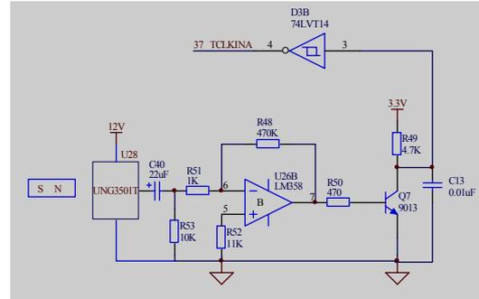
Figure 3. The counter module circuit.
