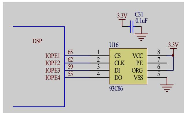
Figure 1. The circuit principle diagram of memorizer.
