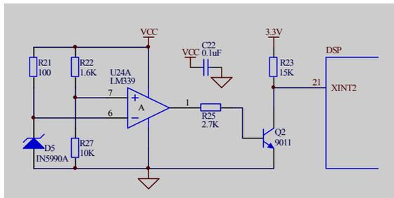
Figure 2. The power detection circuit.
