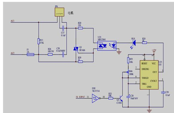
Figure 4 The shaking and alarm circuit.
