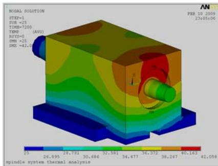
Figure 3. The temperature field distribution of spindle system after modification
