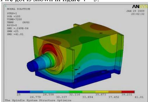
Figure 4. The temperature field distributions after the optimization of spindle system structure
