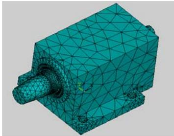
Figure 2 The finite element model of spindle system
