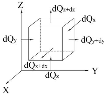
Figure 1. Infinitesimal body's thermal conductivity
