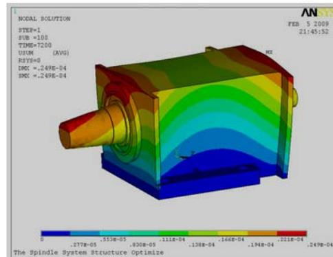
Figure 5. Thermal deformation of spindle system image after optimization
