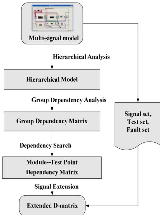
Fig.1 Implementation process from the multi-signal model to extended *D*-matrix
