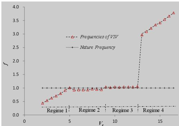
Fig.4 Vibration Frequencies of downstream cylinder of the two cylinders in tandem
