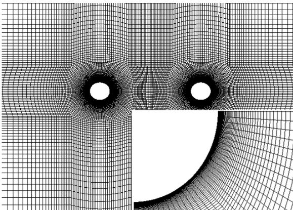
Fig.2 Local mesh near the cylinder
