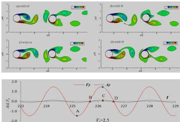
Fig.7 Instantaneous vorticity contours at  $V_r=2.5$  of the downstream cylinder
