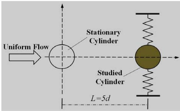
Fig.1 Sketch of two circular cylinders in tandem
