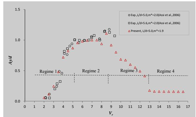
Fig.3 Variation of the reduced amplitude  $A_y/d$  versus reduced velocity  $V_r$  for the downstream cylinder
