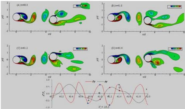
Fig.9 Instantaneous vorticity contours at  $V_r=10.5$  of the two cylinders in tandem
