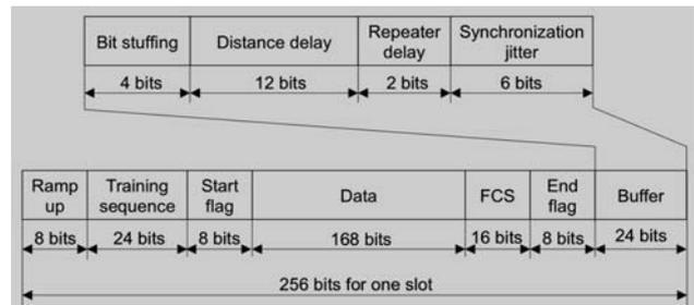
Fig.1 AIS Message Buffer Structure [9]
