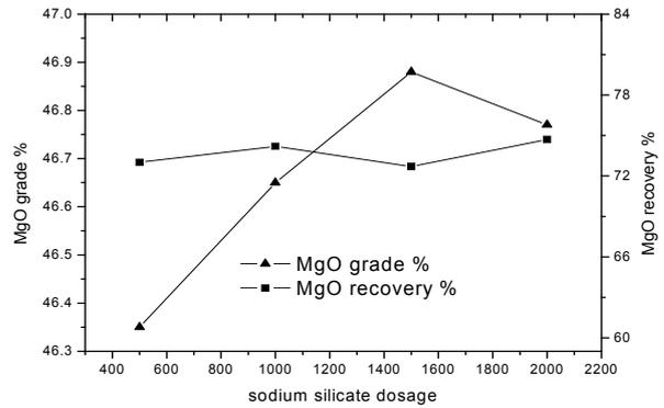
Fig. 6 Dosage of sodium silicate test results.
