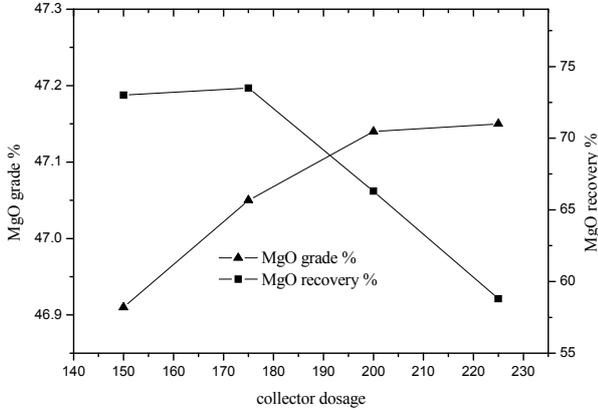
Fig. 7 Dosage of collector test results.
