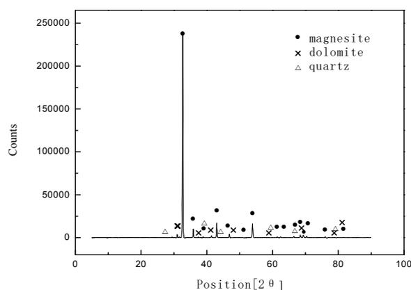
Fig. 1 X-ray diffraction spectrum of magnesite ore.
