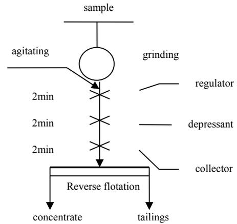
Fig. 2. The flowsheet used for mineral flotation.
