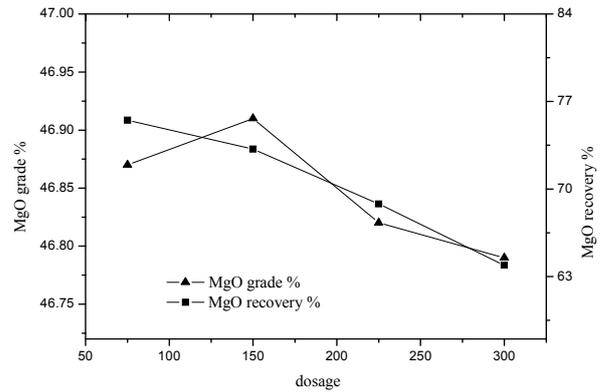
Fig. 5 Dosage of sodium hexametaphosphate test results
