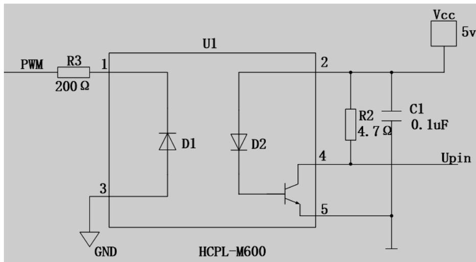
Fig. 2 IPM drive circuit.
