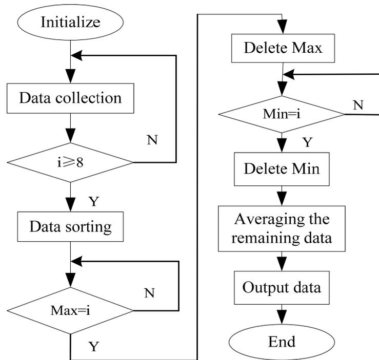
Fig. 3 Flowchart of digital filtering algorithm
