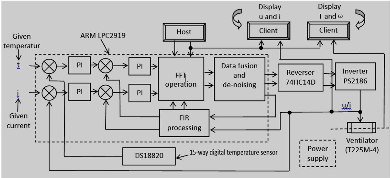
Fig. 4 Experimental control system model
