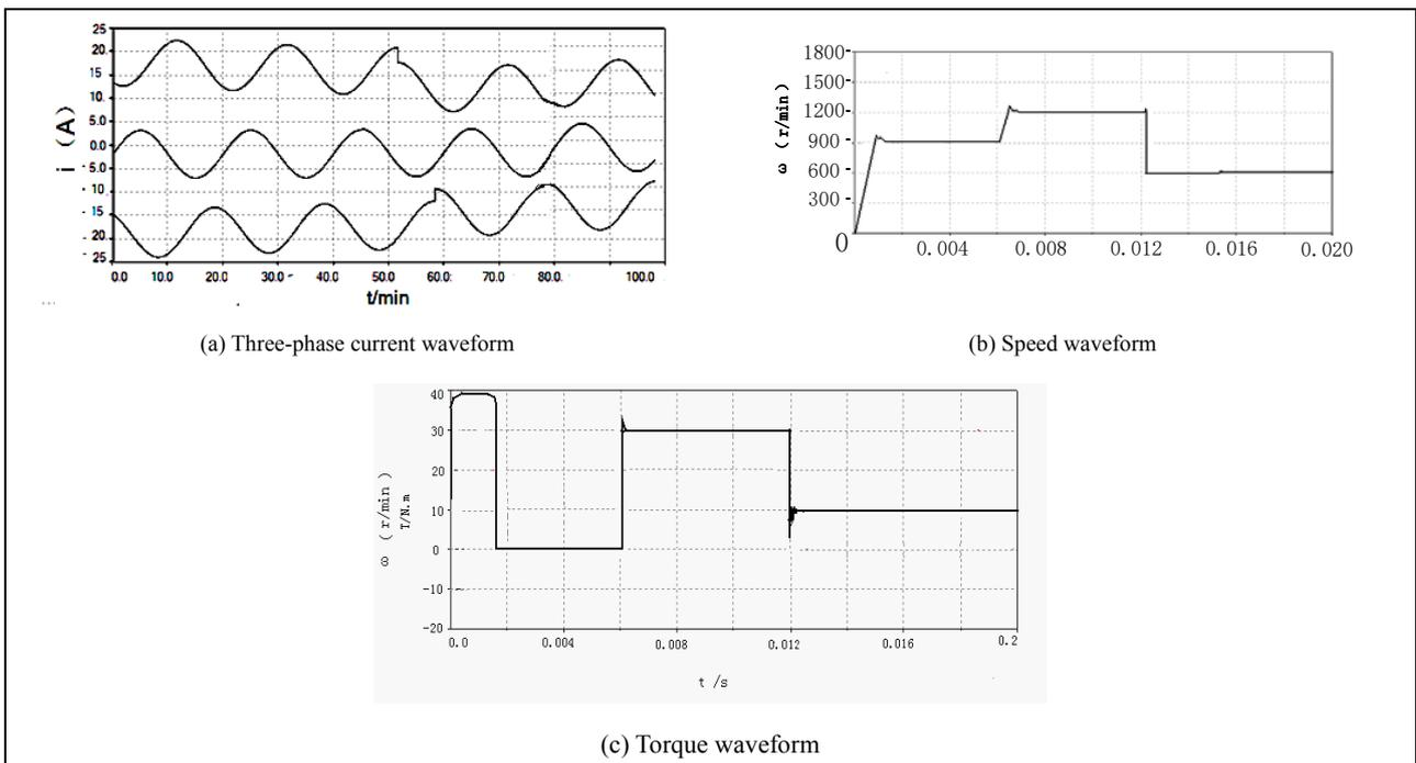
Fig. 6 Operating conditions after fan system optimization
