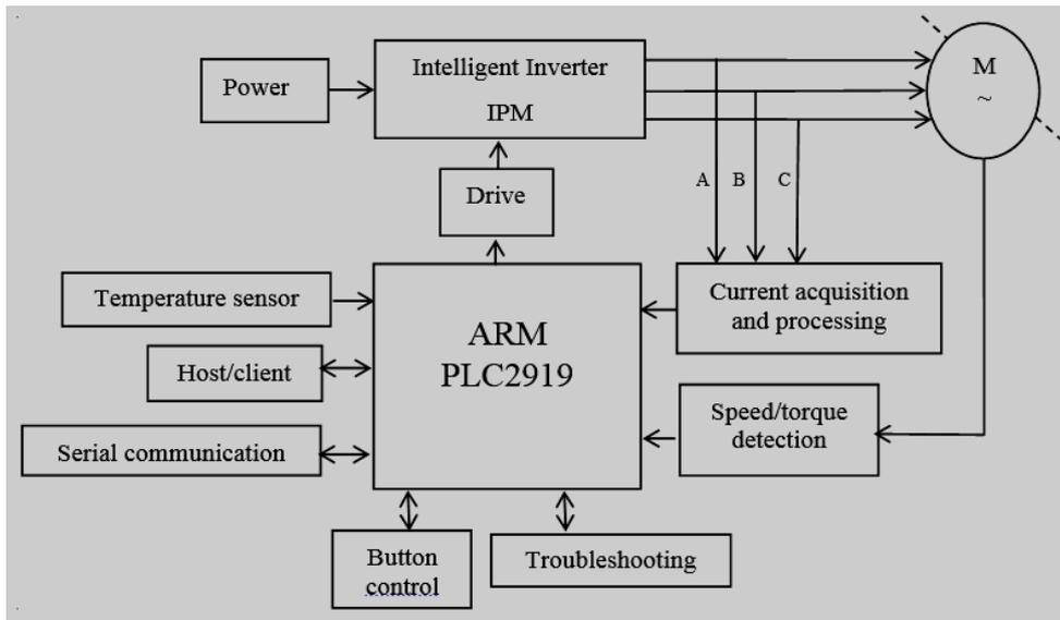
Fig. 1 Block diagram of system hardware configuration.
