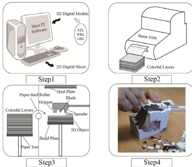
Fig.2 The Printing Process of the Matrix 300A
