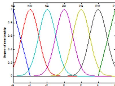
Fig5.  $K_p, k_i, k_d$  Membership Function Curve
