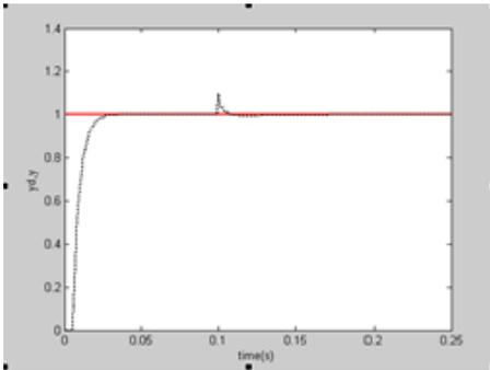
Fig7. Add Interference Unit Step Response of The Fuzzy PID Control.
