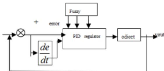
Fig 3 .Parameter Adaptive Fuzzy PID Control System Structure.
