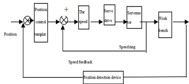
Fig.1. The Structure of Servo System Block Diagram.
