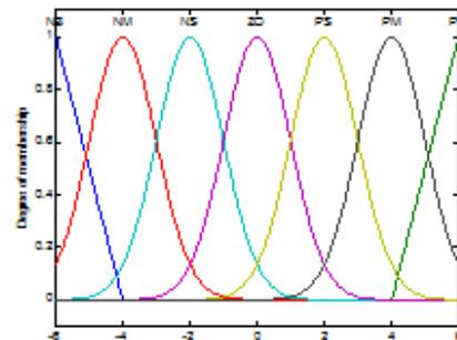
Fig.4. E, EC Membership Function Curve
