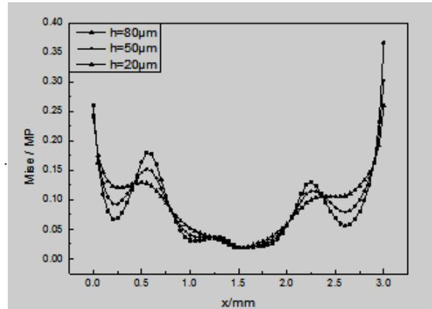
Fig. 6 The distribution along x-axis of the Mises stress with different micro pit depth.
