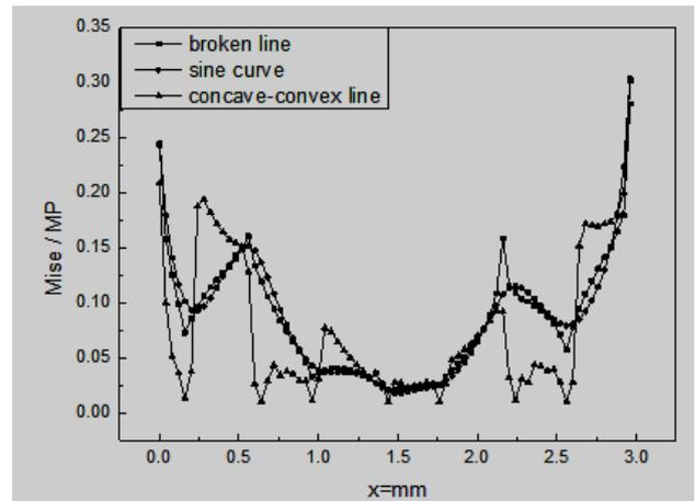
Fig. 9 The distribution along x-axe of the Mises stress with different micro pit morphology.
