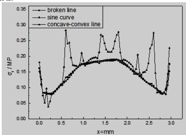
Fig.11 The distribution along x-axis of  $\sigma_y$  of y-axis with different micro pit morphology.
