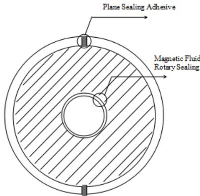
Fig 1 The radial section at the pole shoe of the split magnetic liquid sealing structure
