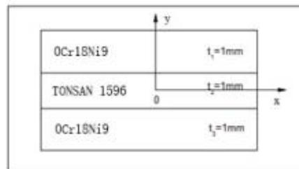
Fig.2 Schematic diagram of the model of matrix and glue coating and matrix
