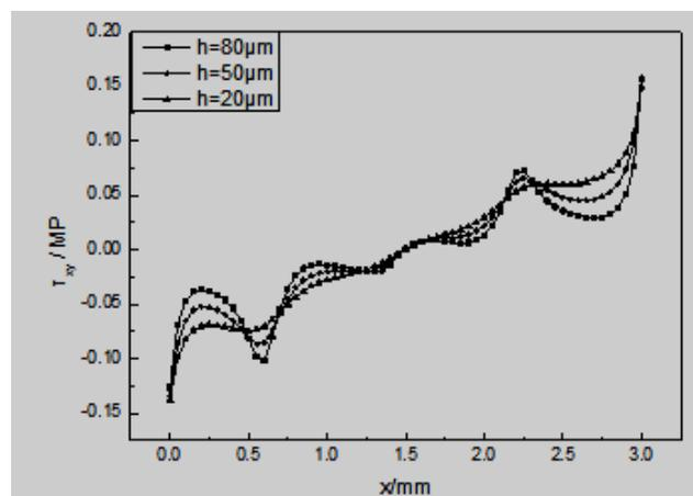
Fig.7 The distribution along x-axis of the shear stress  $\tau_{xy}$  with different micro pit depth.
