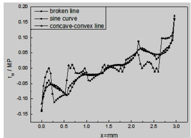
Fig.10 The distribution along x-axe of the shear stress  $\tau_{xy}$  with different micro pit morphology.
