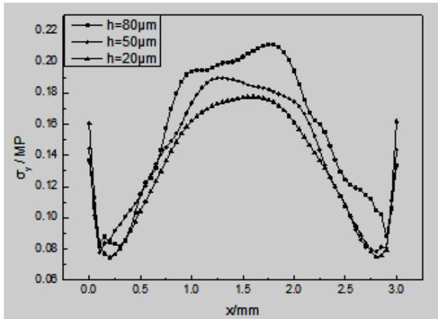
Fig.8 The distribution along x-axe of  $\sigma_y$  of y-axis with different micro pit depth.
