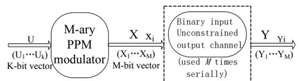
Figure 2. Block diagram of PPM modulator
