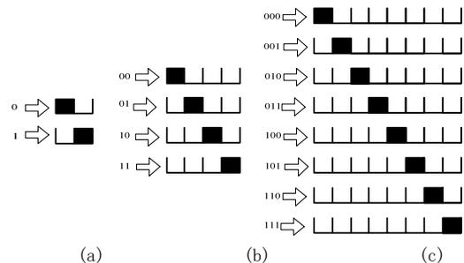
Figure 1.  $M$ -ary PPM maps  $\log_2 M$  bits to a pulse in one of  $M$  positions—(a) binary PPM, (b) 4-ary PPM, (c) 8-ary PPM.
