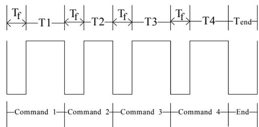
Figure 3. Coding mode of signal transmission system
