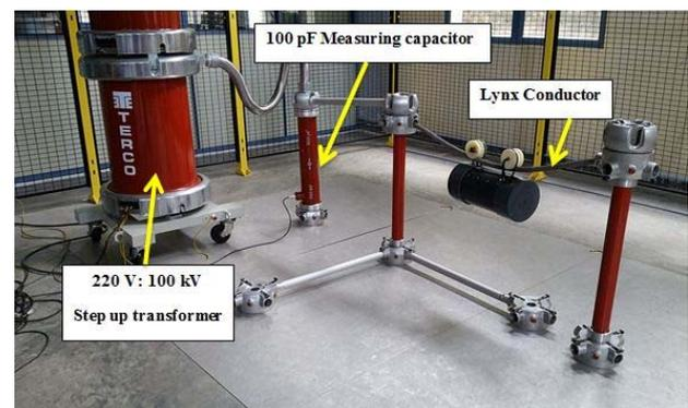
Fig.19. Testing apparatus for electromagnetic shield operation
