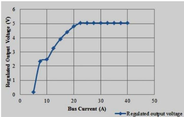
Fig. 9. Experimental output of the developed magnetic energy harvesting circuit for the resistor value of 470 ohms
