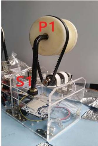
Fig. 3. Arrangement of a single wheel in the ROV prototype
