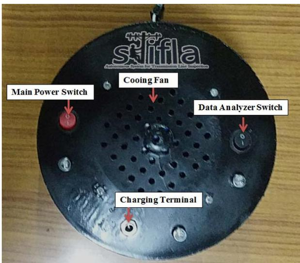
Fig. 7. Back panel of the ROV prototype
