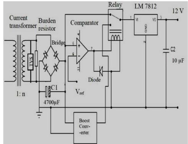
Fig. 8. Magnetic energy harvesting circuit
