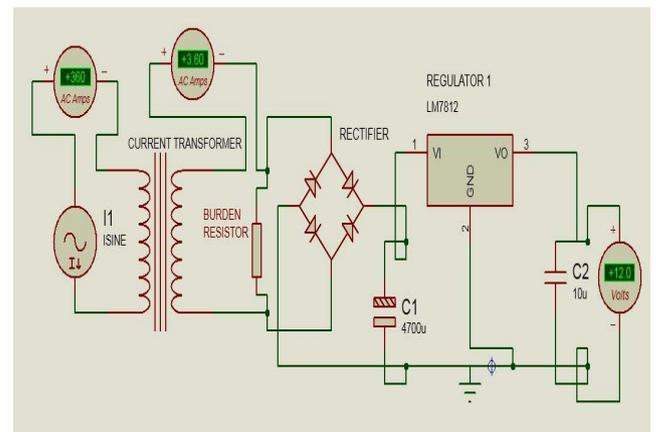
Fig. 11. Simulated magnetic energy harvesting circuit using PROTEUS®
