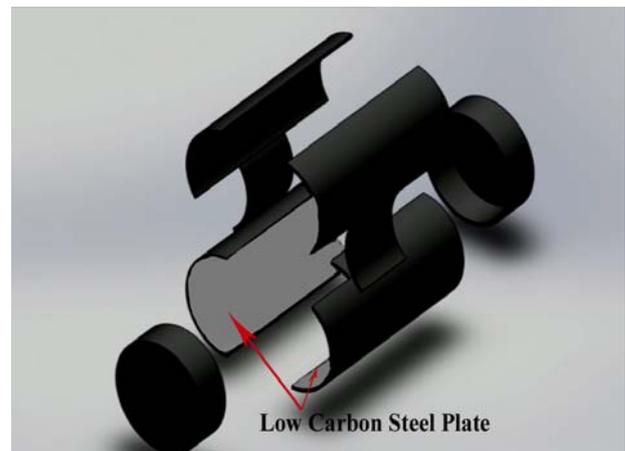
Fig. 4. Magnetic shielding Enclosure of the ROV prototype
