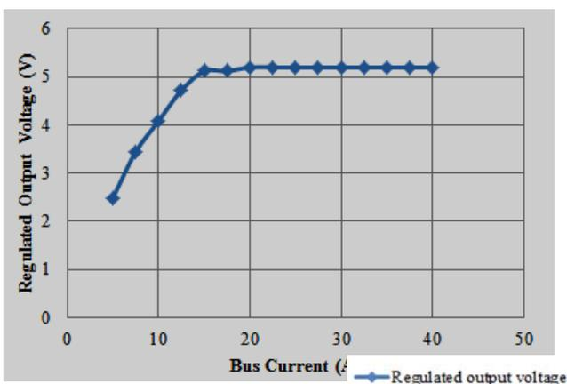
Fig. 10. Experimental output of the developed magnetic energy harvesting circuit for the resistor value of 1000 ohms
