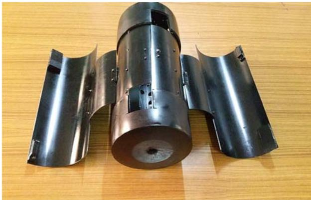
Fig. 6. The complete enclosure of the ROV prototype
