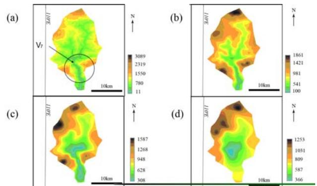
Fig. 6. Elevation, 2nd -3rd order, 3rd – 4th order and 4th – 5th order streams isobases maps of the northern drainage basin
