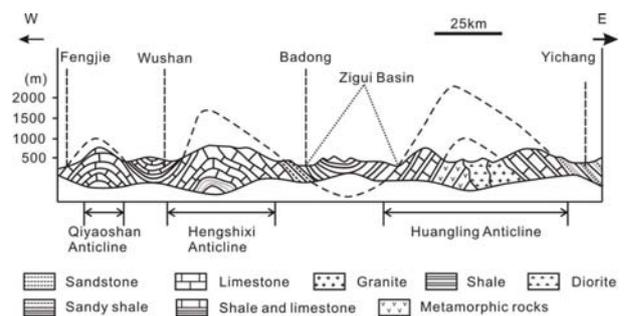
Fig. 12. Asymmetry of the Hengshixi Anticline.
