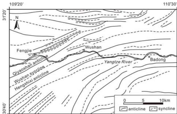
Fig. 3. Map of the different anticlines and synclines of the Three Gorges area.
