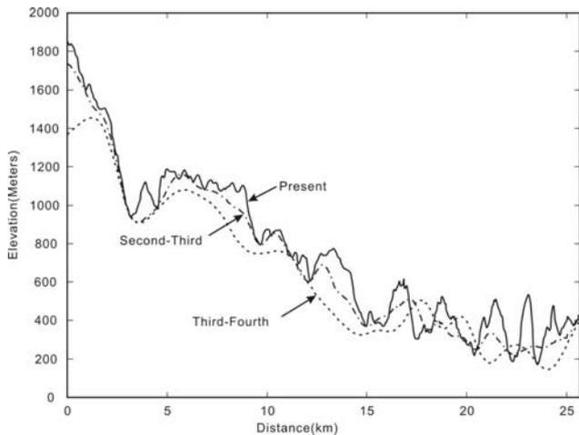
Fig. 8. Elevation profile of current elevation, Second-third isobase surface, and Third-fourth isobase surface.
