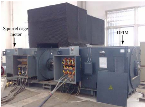
(a) Experimental motors platform
