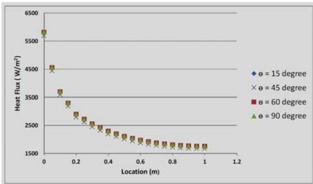
Figure 5. Variations of heat flux with different tilt angles at the convection surface.
