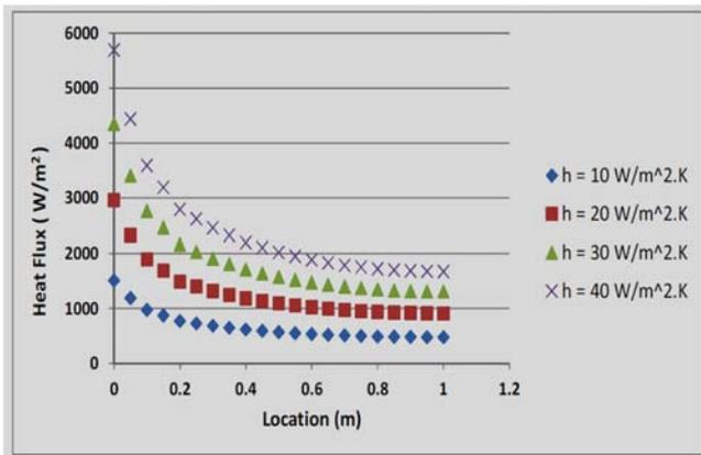
Figure 6. Variations of heat flux with different heat transfer coefficient.
