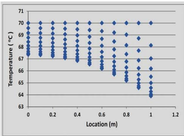
Figure 4. Variations of temperature in the plate.
