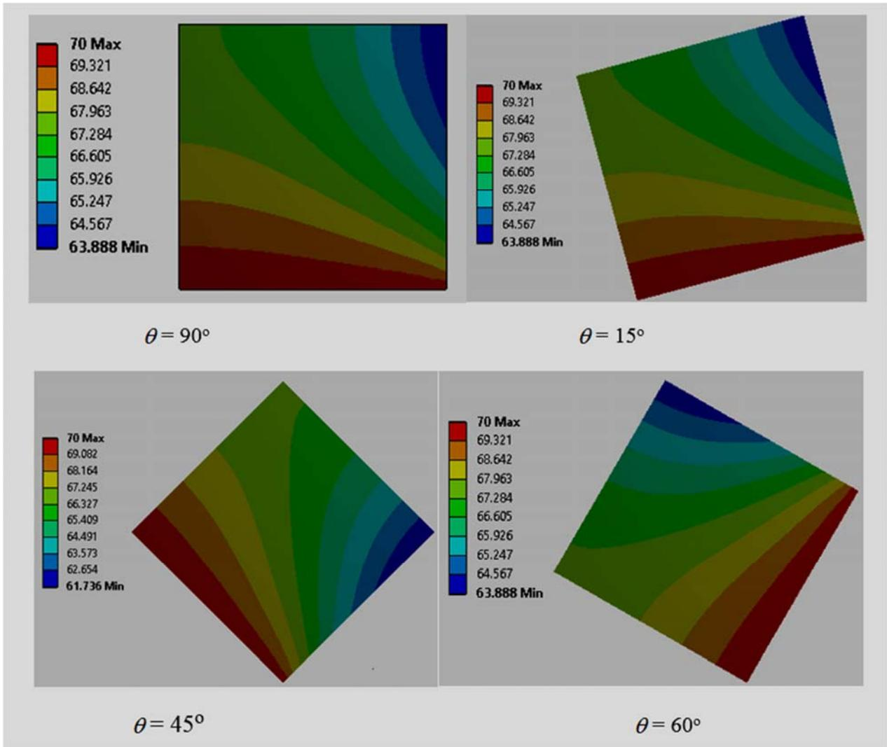
Figure 3. Temperature distribution contour at different  $\theta$  s.
