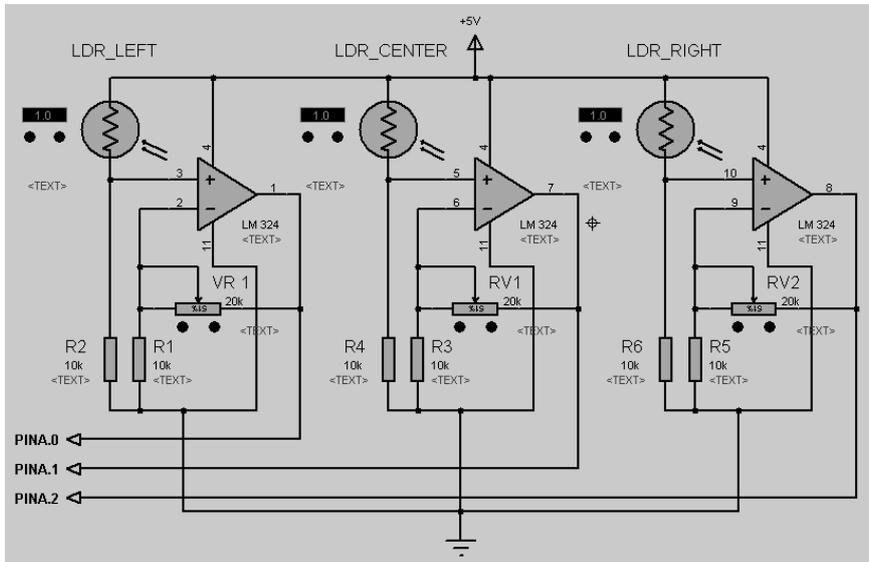
Figure 1. Light sensor circuit.
