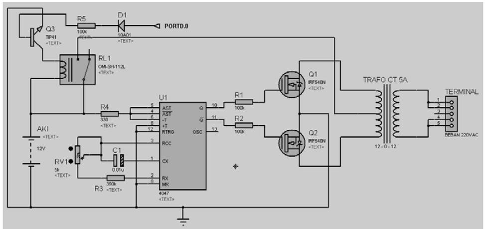
Figure 3. Inverter system of the EPS.
