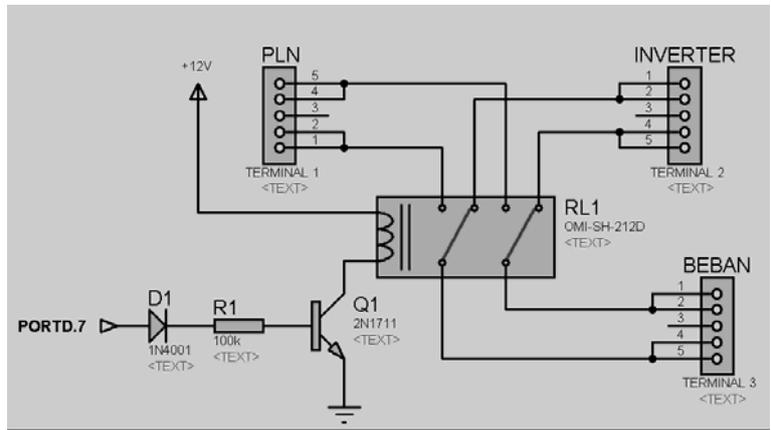
Figure 4. Source Select switch scheme.
