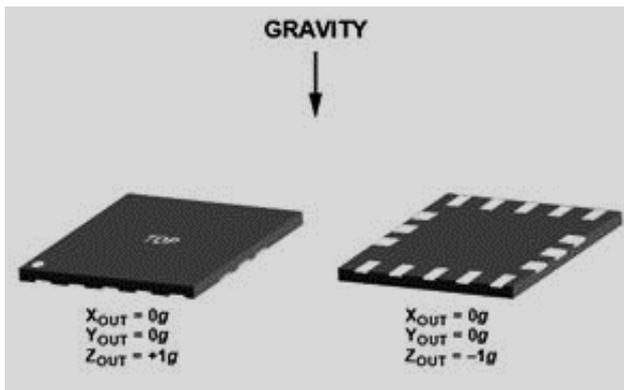
Figure 2. Orientation of Accelerometer in two reading
