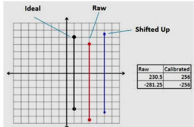
Figure 3. Rescaling and Shifting of Measured Values
