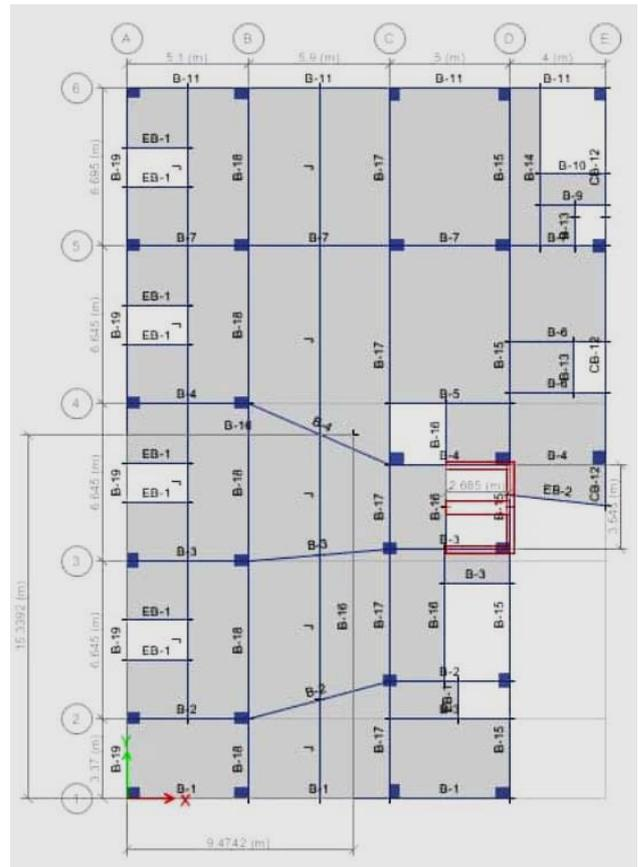
Figure 5. Floor Plan of Roof Deck
