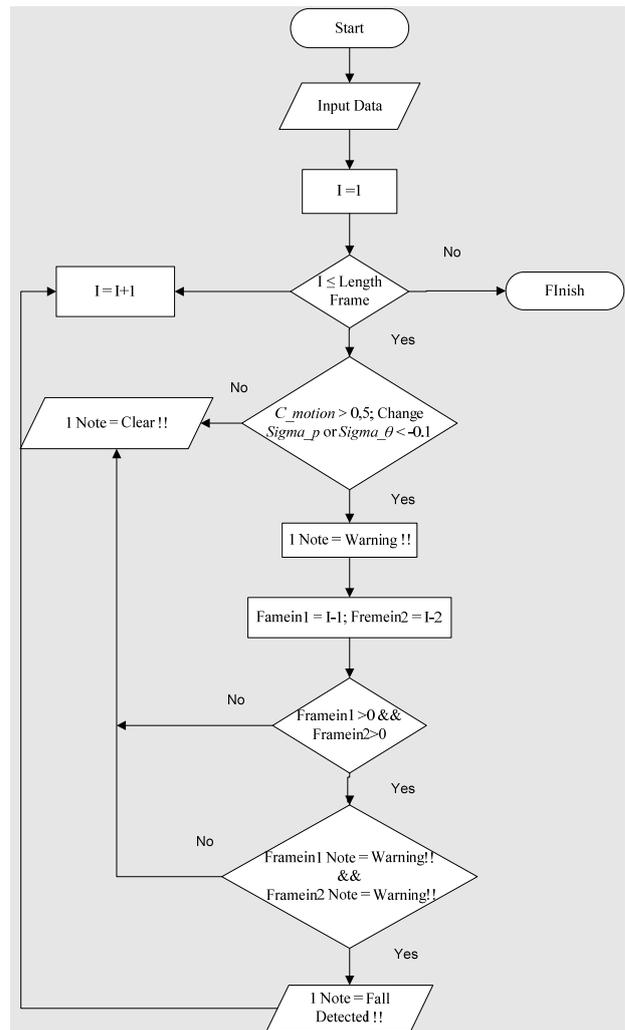
Figure 4. Fall Detection System Algorithm
