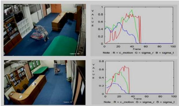
Figure 7. System's response on different fall position
