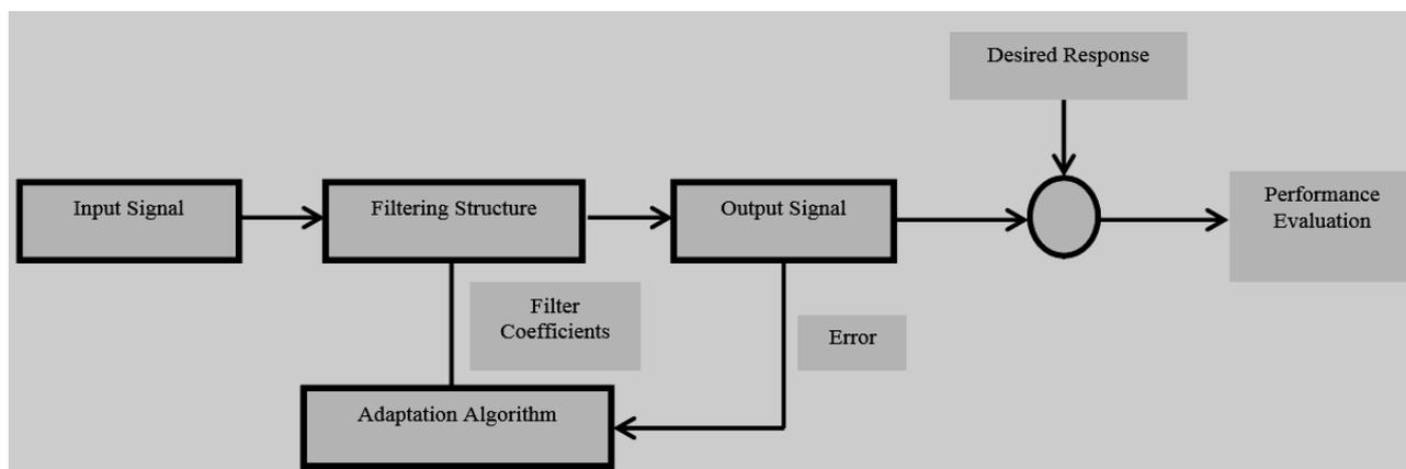
Figure 1. Design system of adaptive filter.
