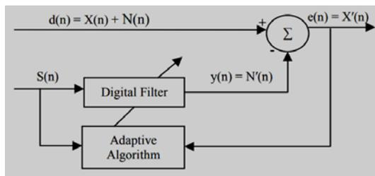
Figure 4. Principle of adaptive filter
