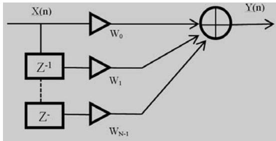
Figure 5. Digital filter structure
