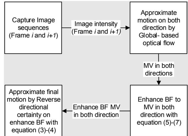
Figure 1: Process flow of B-R
