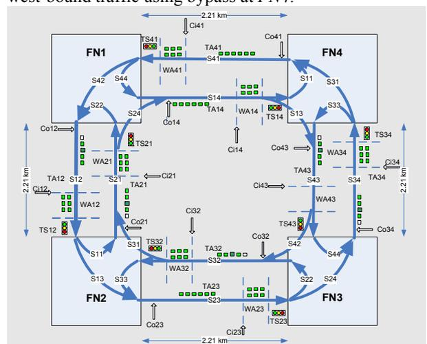
Figure 7. Identification of Main Road (S), Bypasses (S), Transition Areas (TA), Waiting Areas (WA), Counters (C), and Traffic Signals (TS).
