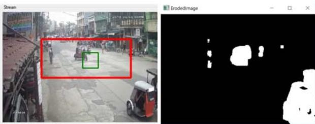
Figure 2. Boundary Perspective in Camera View (Vehicle Counter)
