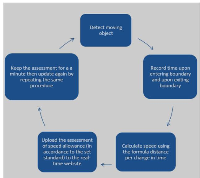
Figure 3. Procedure on Speed Assessment
