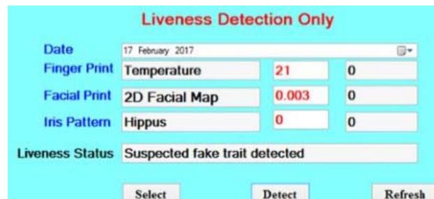
Figure 5: Screenshot of 5<sup>th</sup> instance of Liveness Detection simulation showing detection of suspected fake trait.
