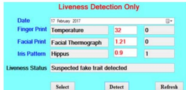
Figure 3: Screenshot of 1<sup>st</sup> instance of Liveness Detection simulation showing detection of suspected fake trait.
