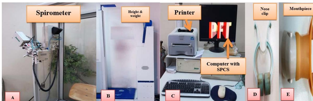
Fig. 2: Spirometer with the requirement of PFT (A) spirometer (B) weight and height scale (C) computer with SPCS software and printer (D) nose clip (E) mouthpiece
