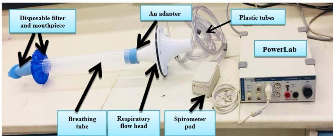
Fig. 1: PowerLab (26T) with spirometry
