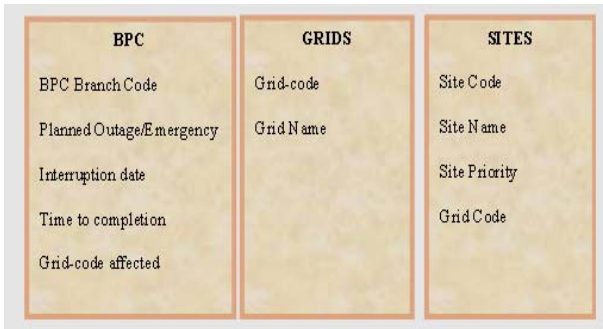
Figure 3. Table planning on the required tables to create a database with. Three (3) required tables include: BPC table, Grids table and Sites table.
