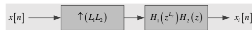
Figure 4(c). The identified block diagram of the one state up-sampling concept for two state up-sampling process.
