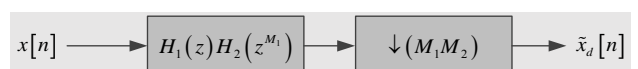
Figure 3(c). The identified block diagram of the one state down-sampling concept for two state down-sampling process
