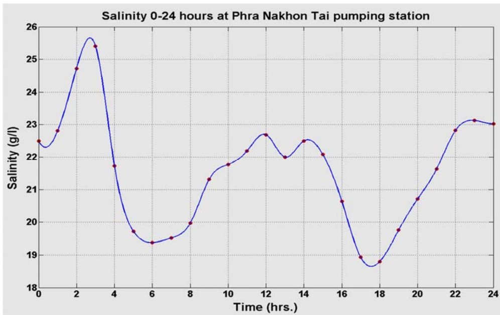
Figure 3. Cubic spline interpolated left boundary condition S(0,t) (g/l) (the left boundary was the sea)
