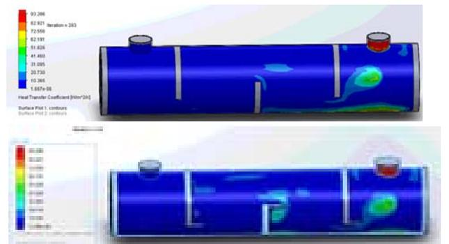
Figure 10. Cut Plane Heat Transfer Coefficient of Shell
