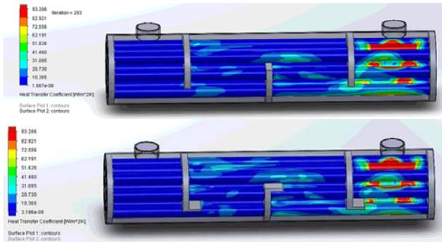
Figure 11. Cut Plane Heat Transfer Coefficient of Tube
