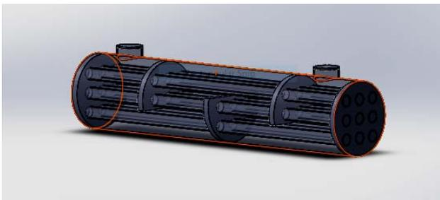
Figure 3. Assembly of SB-STHE
