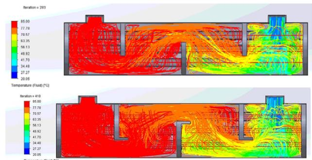
Figure 6. Fluid Flow Simulation
