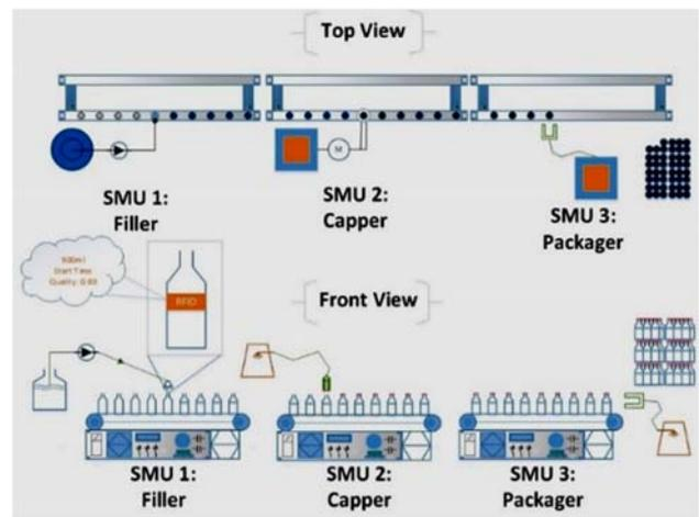
Figure 5. Water Bottling Production Line
