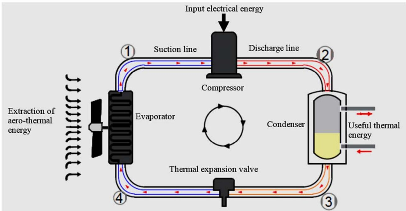
Figure 1. A schematic block diagram of the main components of an ASHP
