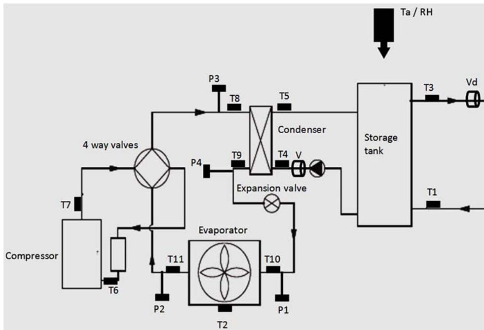
Figure 5. Schematic layout of the installed split type ASHP water heater and the sensors
