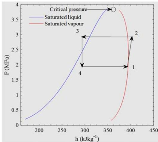
Figure 3. P-h graph of the VCRC in ASHP water heater using R417A
