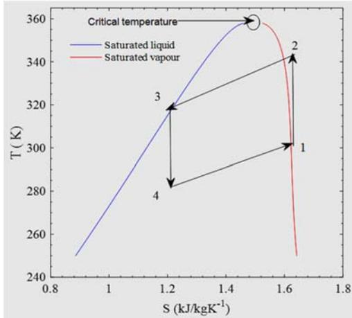
Figure 2. T-S graph of the VCRC in ASHP water heater using R417A
