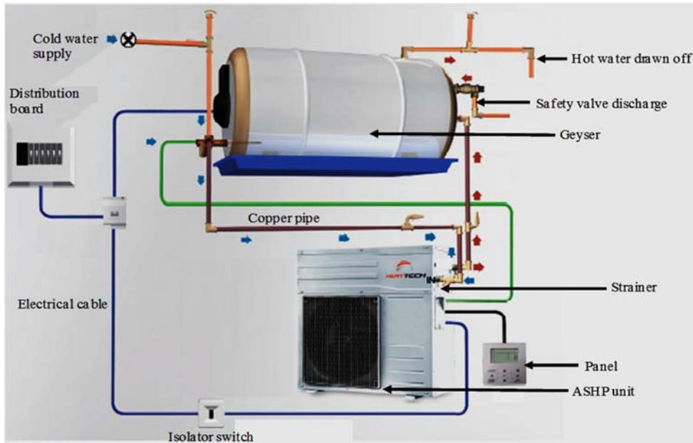
Figure 4. Schematic diagram of the installed split type ASHP water heater
