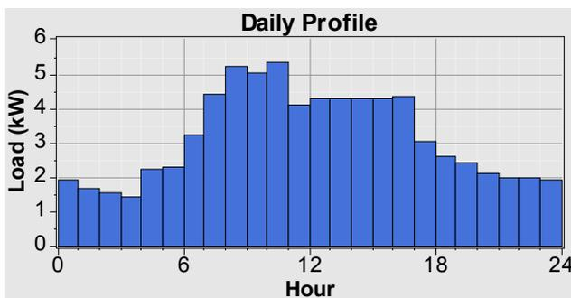
Figure 2. Load profile of a typical farm [2]
