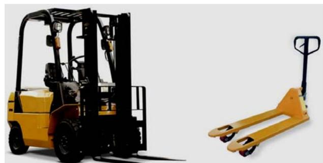
Fig. 2. The two types of vehicles for the transportation of pallets: forklift and trans-pallet.
