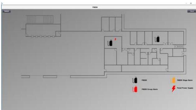
Figure 20. GUI of FM200 system in the station.
