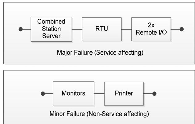
Figure 10. SMS model RBD for major and minor failures.
