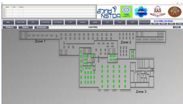
Figure 15. GUI of the lighting system operation.
