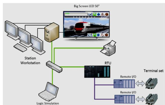
Figure 2. Diagram of the computer system architecture.
