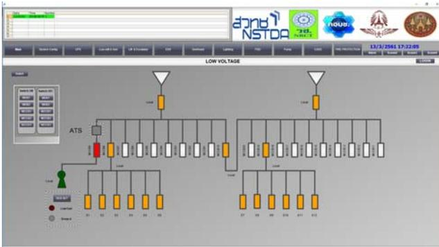
Figure 14. GUI of the low-voltage power supply system.
