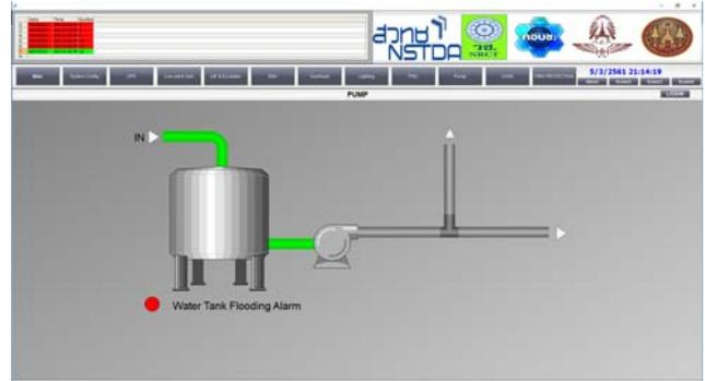
Figure 21. GUI of the water pump system during an alarm.
