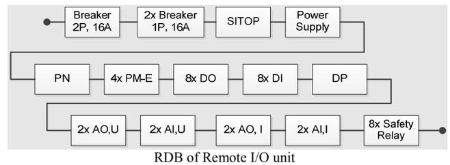
2) *RTU Unit:* Similar to the Remote I/O, the failure of a single set of remote I/O subsystems can be arranged in a series configuration per Fig. 6.
