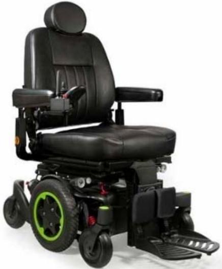
Figure 2. Mobile wheelchair with two differential-drive motors.
