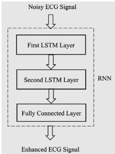
Figure 1. The schematic diagram of RNN algorithm used in this paper.
