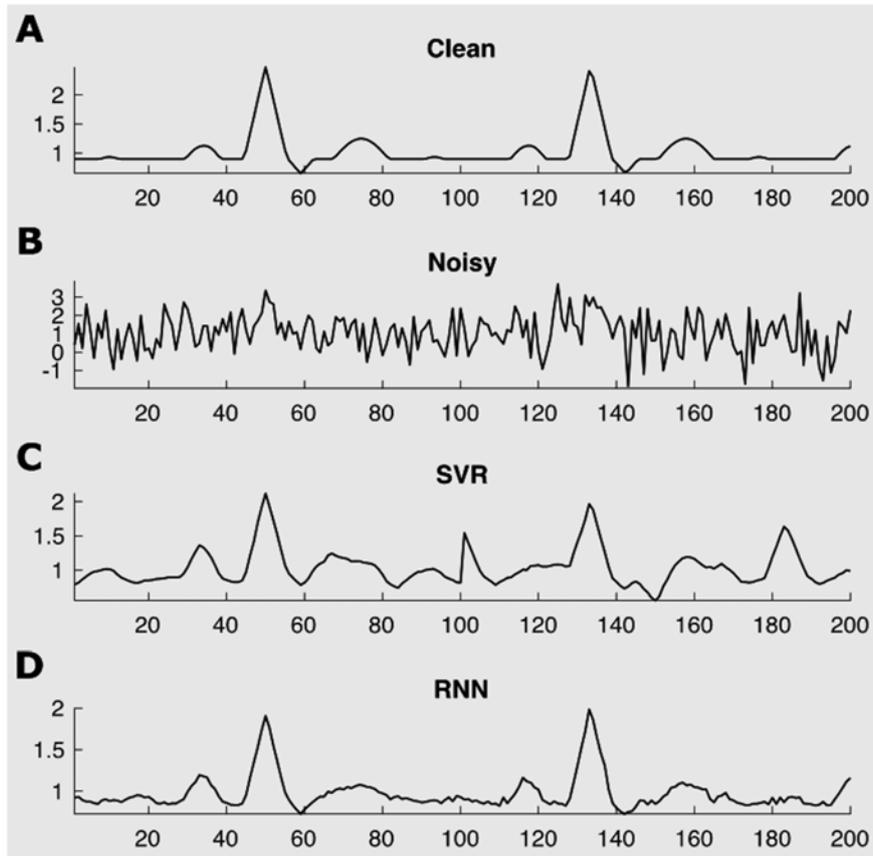
Figure 3. An example of (A) clean ECG signal (200-time samples or two frames), (B) noisy signal with SNR = 1 dB, (C) noisy signal processed by SVR, and (D) noisy signal processed by RNN.
