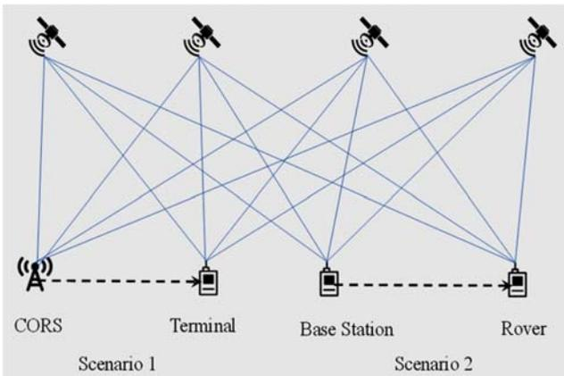
Figure 1. The two basic scenarios of high accuracy GNSS positioning.
