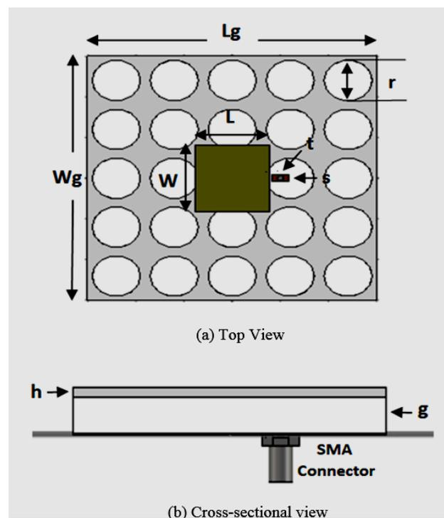
Fig. 1. Rectangular patch antenna with capacitive feed.
