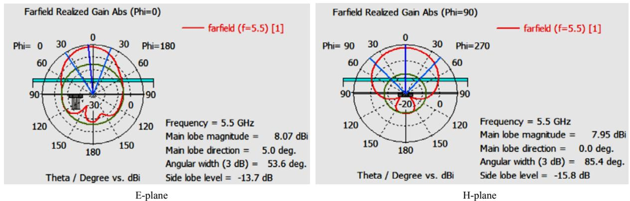
Fig. 4. E-plane and H-plan radiation patterns of the proposed antenna.
