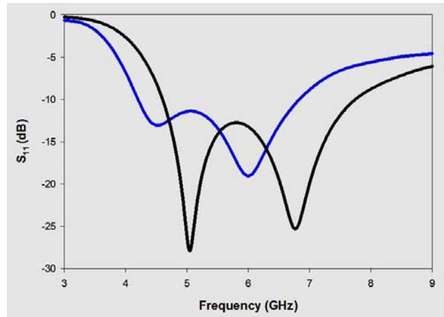
Fig. 2. Input impedance of the proposed antenna with and without air holes.
