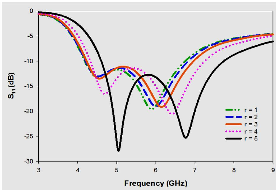
Fig. 3. Effect of changing the radius of the air holes.
