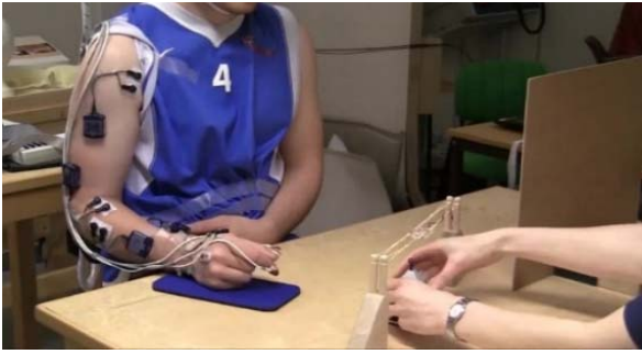
–Figure 5. The experimnet details. Dataset was collected from (12 subjects) with each having 328 trials which resulted in a total of 3,936 grasp and lift trials. Picture source: Luciw et. al. [18].
